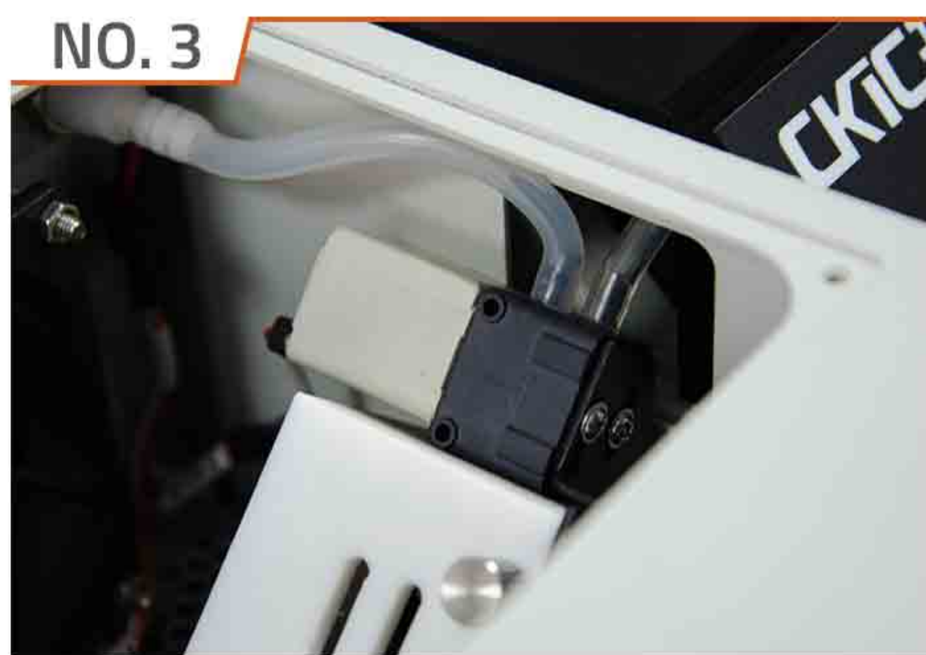
NO. 3 Unique three valve design to avoid cell contamination
