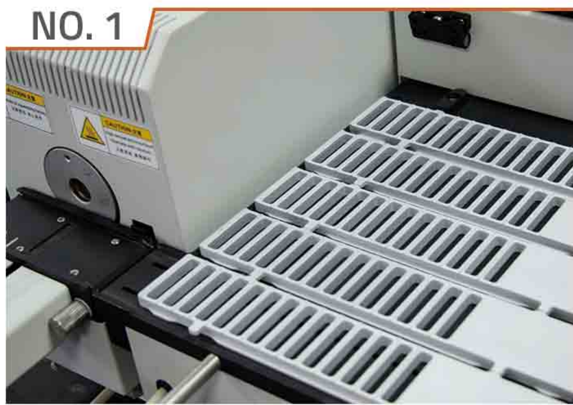
NO. 1 70 position auto-sampler for high sample throughput
